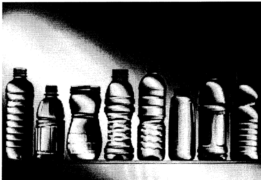
Polypropylene can offer some material advantages such as lower density in blowmolded containers and hot-fill capability that competitive resins such as PET, polystyrene, or vinyl don't provide.
